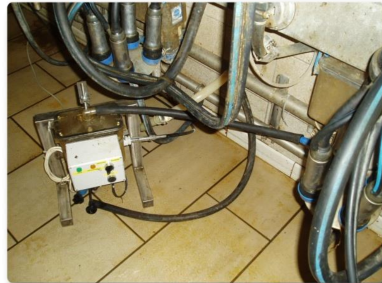
Figure 2 : NIR automatic on-line recording device installed at the CRA-W milking parlour.
